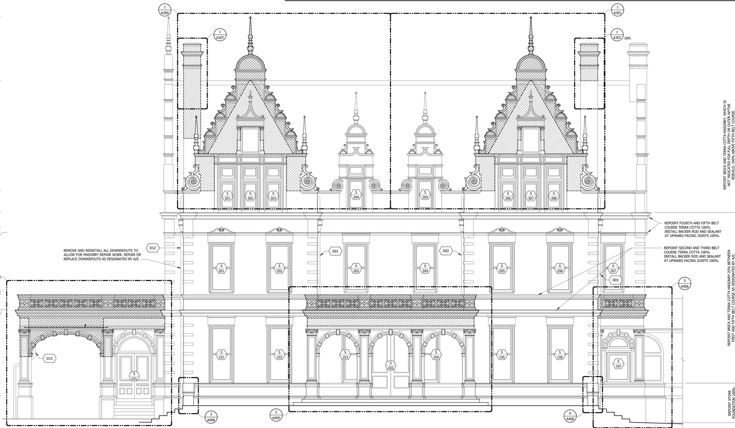
REMOVE AND REINSTALL ALL DOWNSPOUTS TO ALLOW FOR MASONRY REPAIR WORK. REPAIR OR REPLACE DOWNSPOUTS AS DESIGNATED BY A/E.
