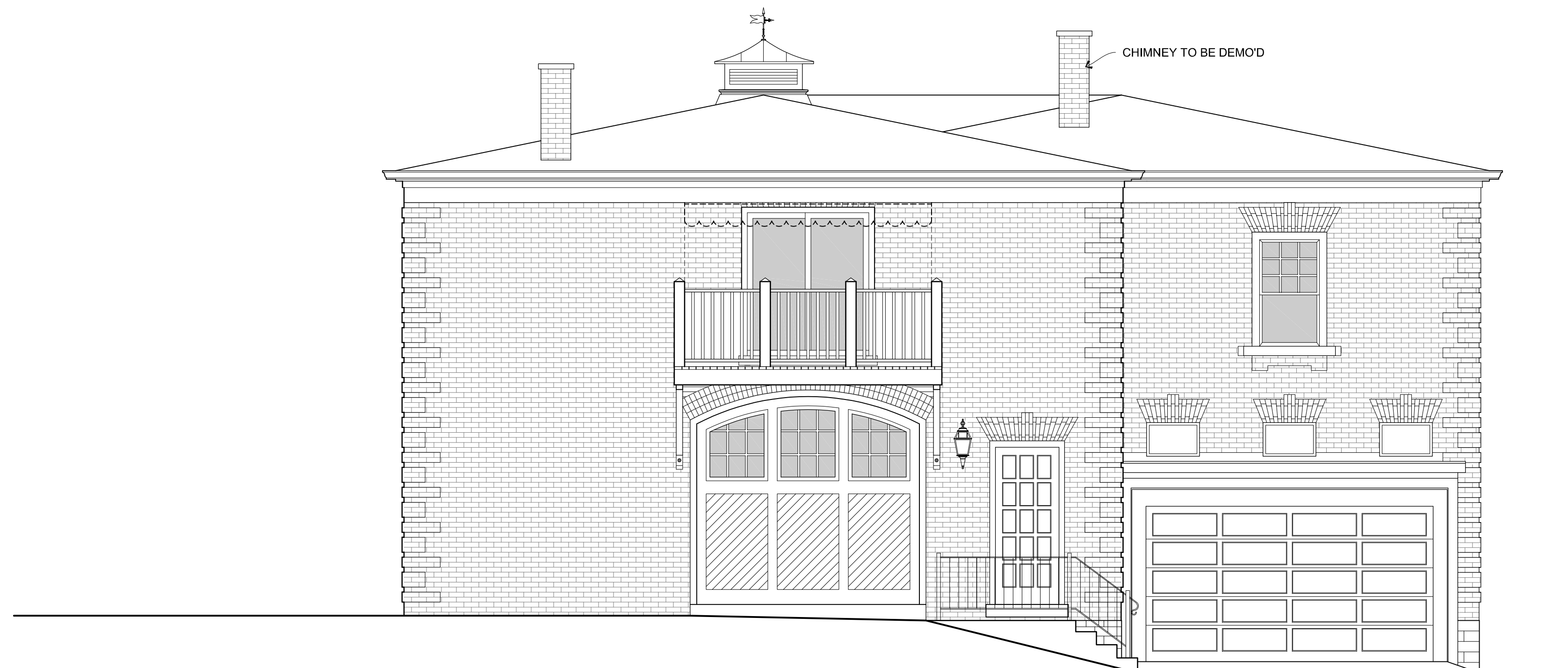
3 EXISTING EAST BUILDING ELEVATION SCALE: 1/4" = 1'-0"
