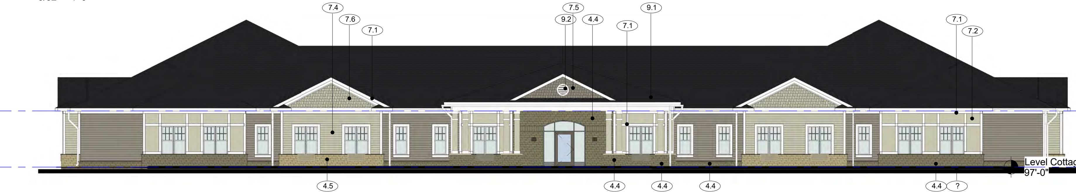
5 Exterior Elevation - Phase II - South 3/32" = 1'-0"
