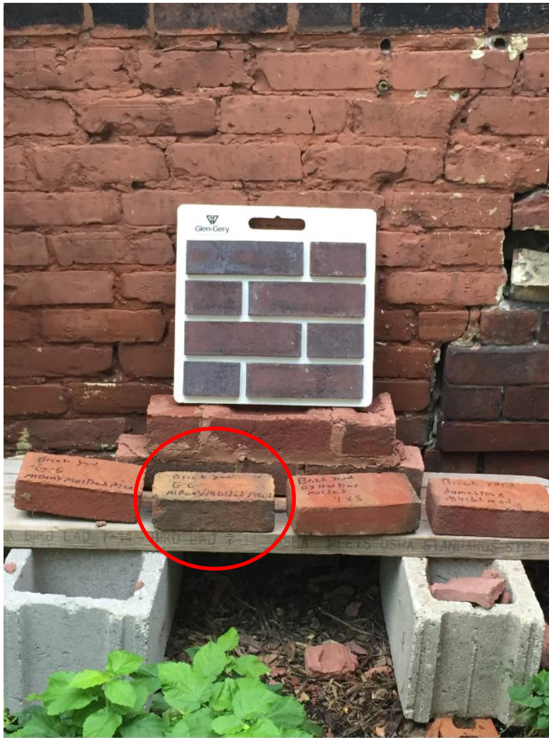
Detail images of (Left) the mortar sample, coursing sample (indicating Flemish bond) and (Right) brick to be utilized for infill at this location and for the reconstruction of the southern chimney
