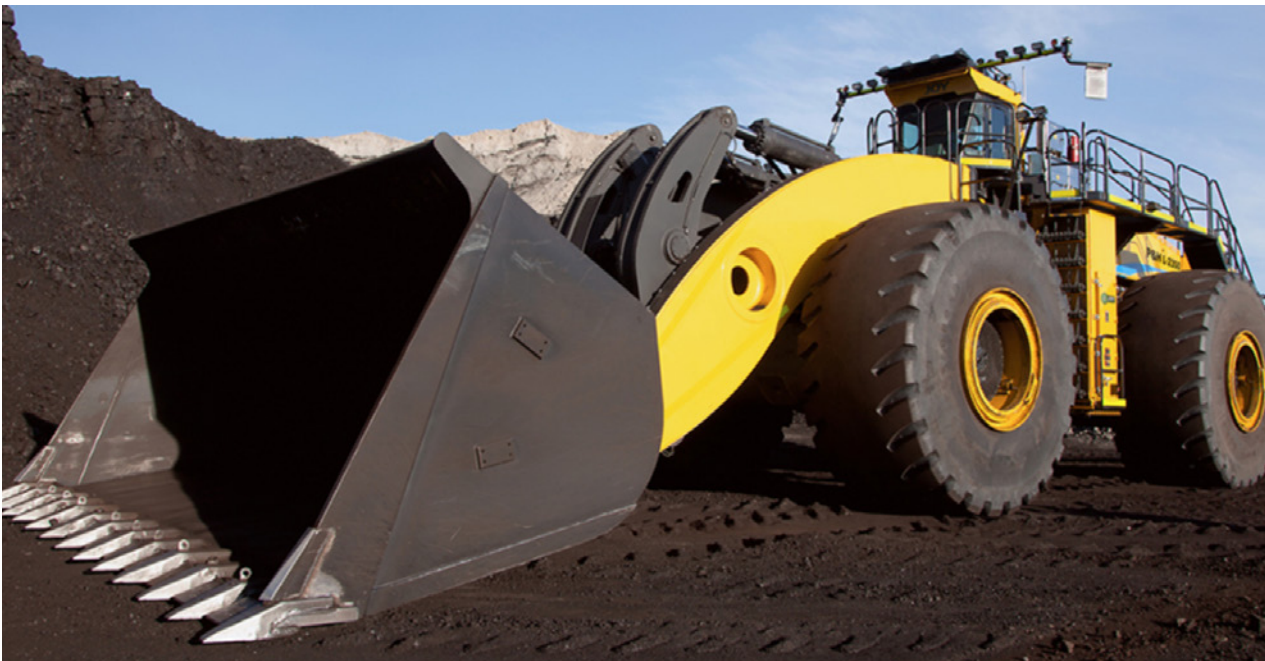
P&H-brand L-2350 wheel loader features the standard bucket capacity of 40.52m 3 , about doubling that of KOMATSU-brand WA1200 wheel loader, the largest model conventionally offered by Komatsu.
