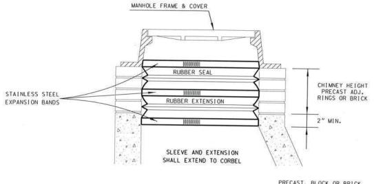
PRECAST, BLOCK OR BRICK MH CONE/CORBEL
