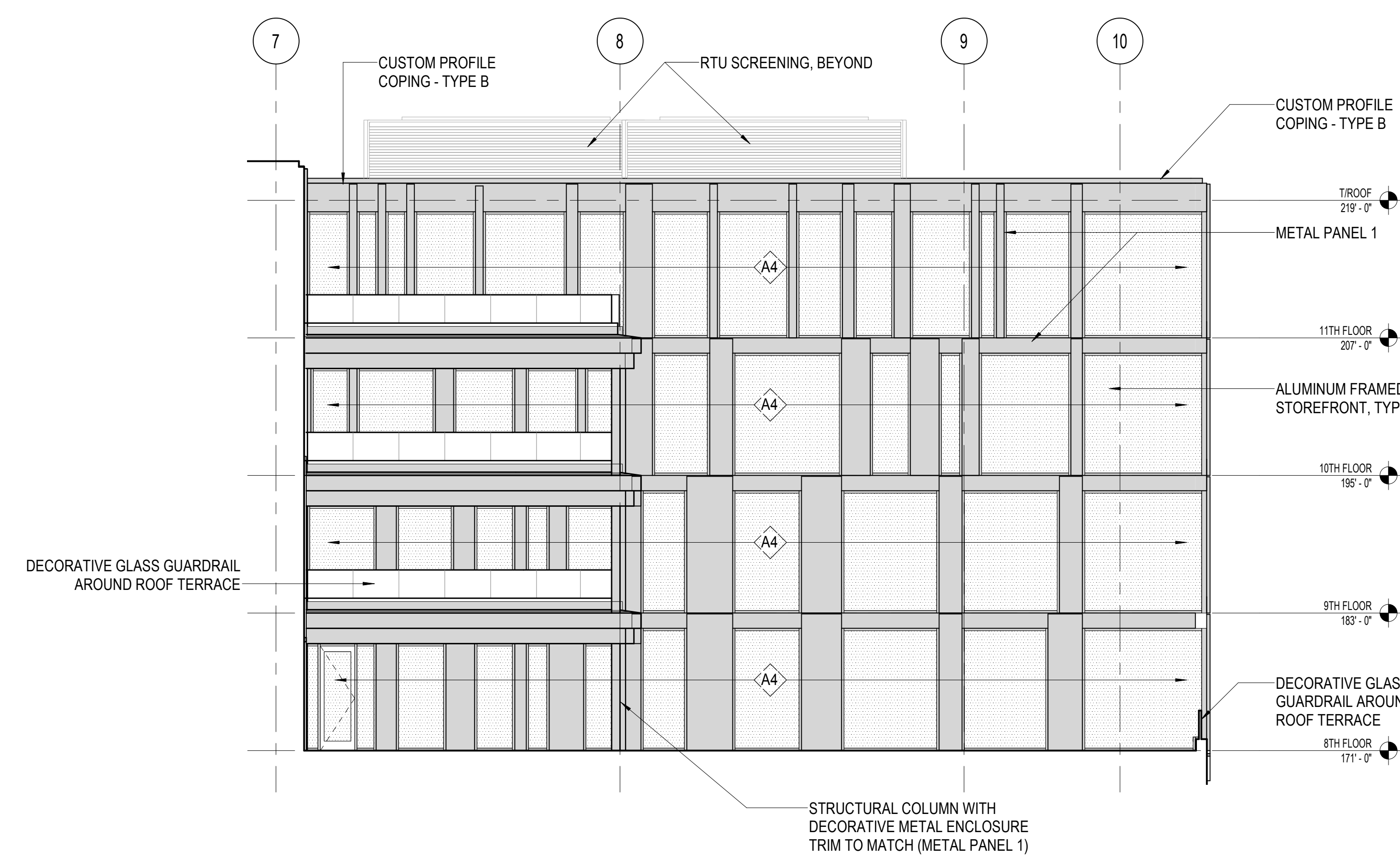
3 PARTIAL EAST ELEVATION - TERRACE SCALE: 1/8" = 1'-0"
