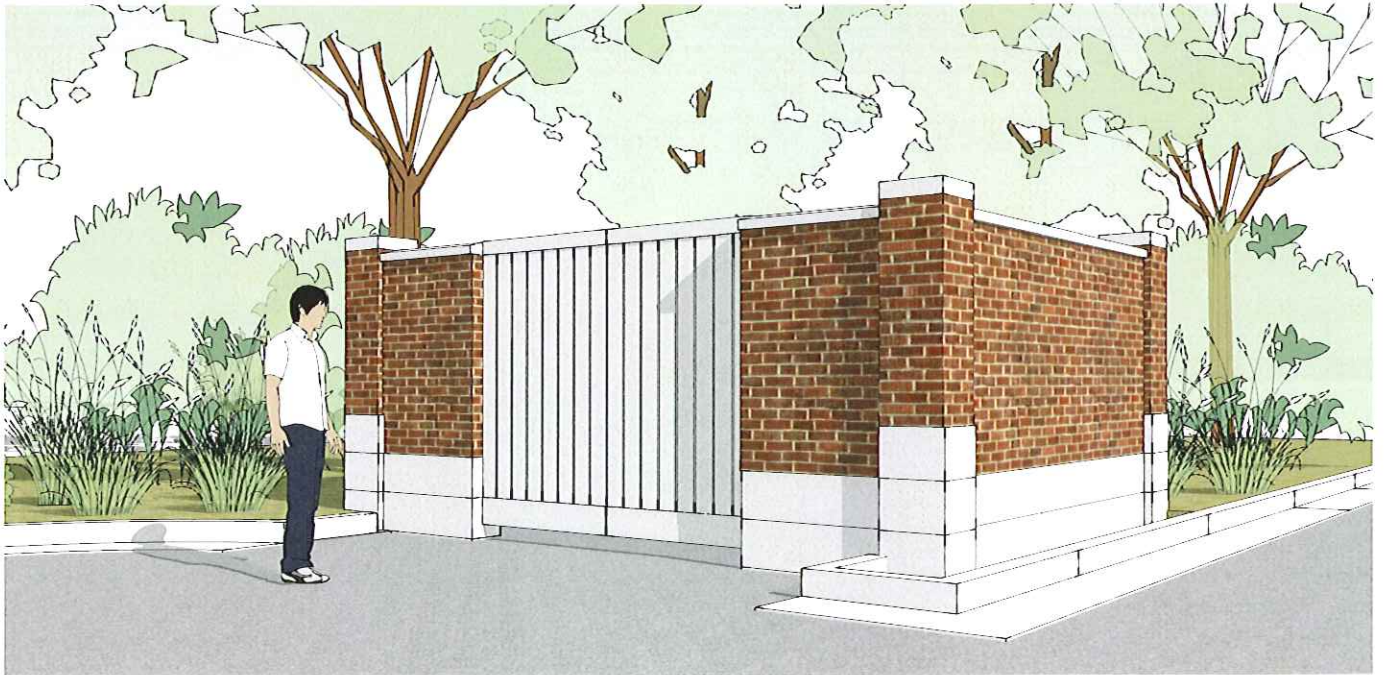
MASONRY SCREEN WALL TRASH ENCLOSURE
