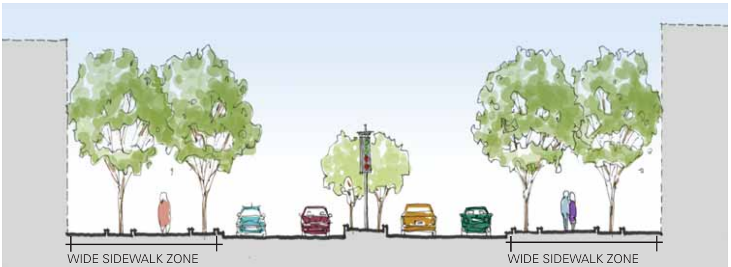
Figure 10.23: North Avenue proposed section showing additional landscaping and widened sidewalks designed to provide traffic calming and make the commercial district more pedestrian friendly.
