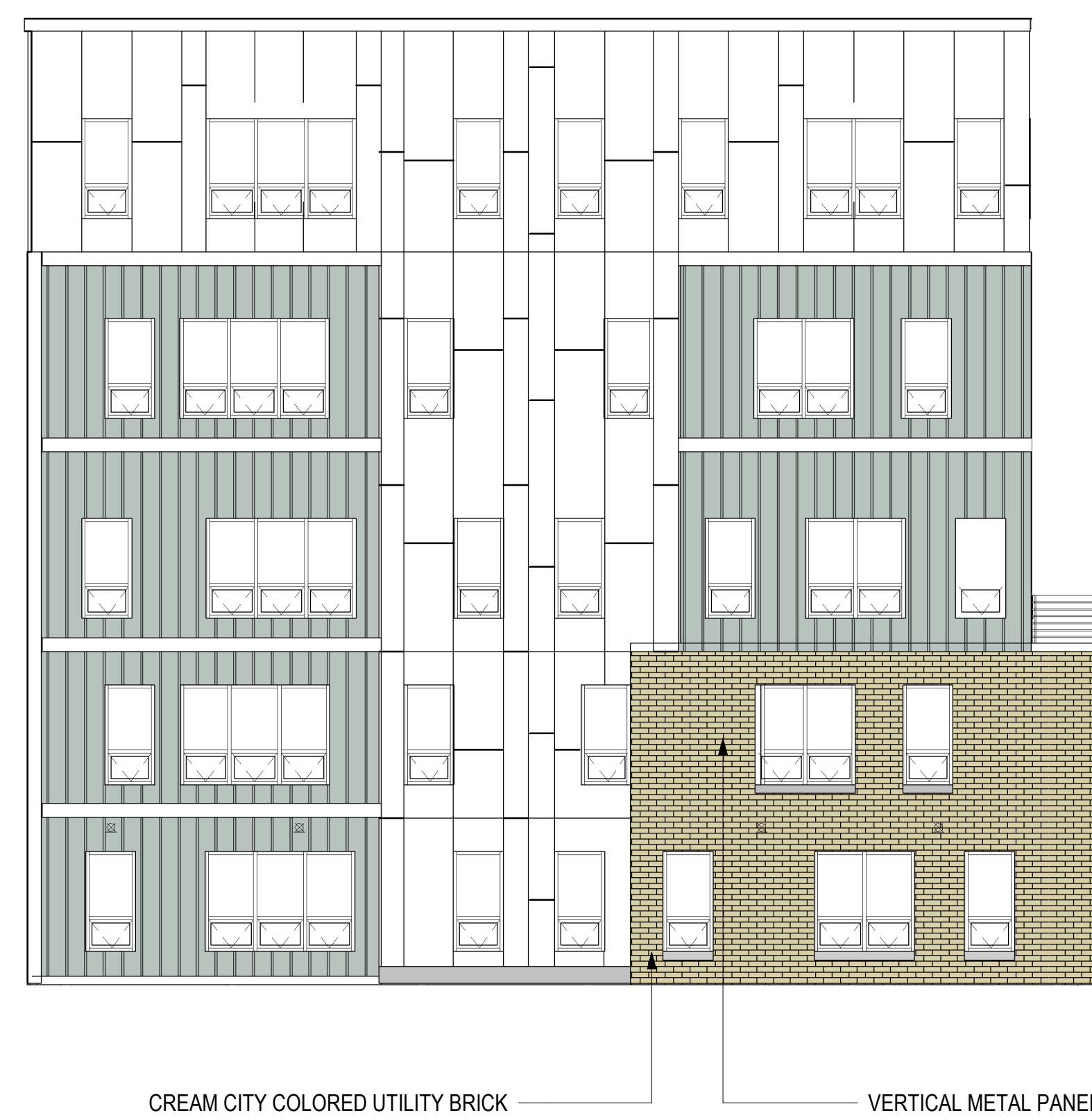
5 NORTH ELEVATION ANGLED WALL Scale: 1/8" = 1'-0" 0' 2' 4' 8' 12'
