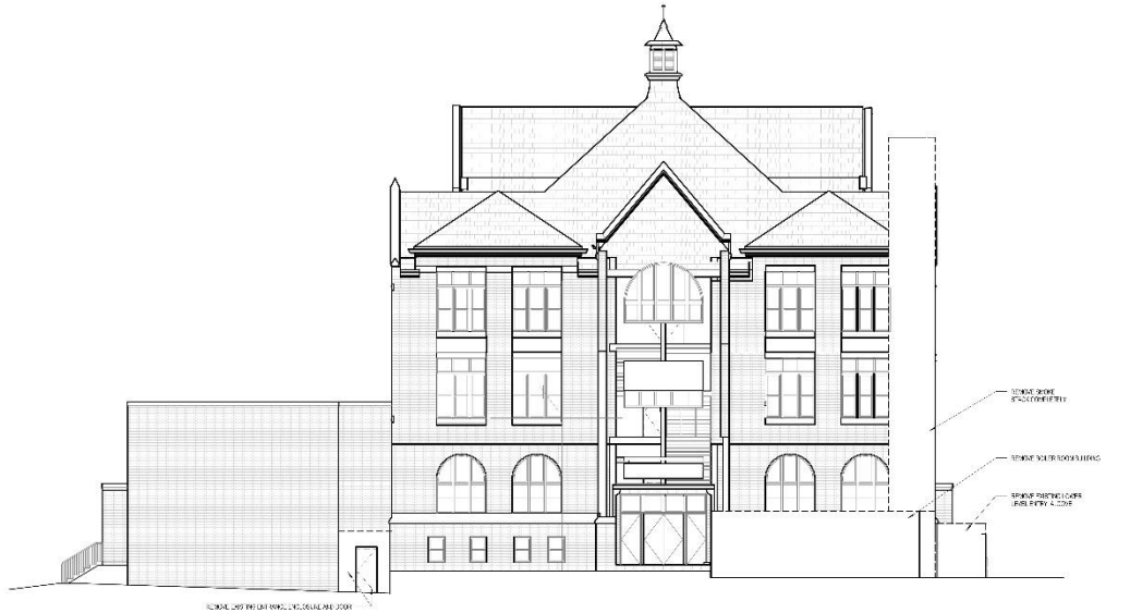
② NORTH DEMOLITION ELEVATION SCALE: 1/8" = 1'-0"
