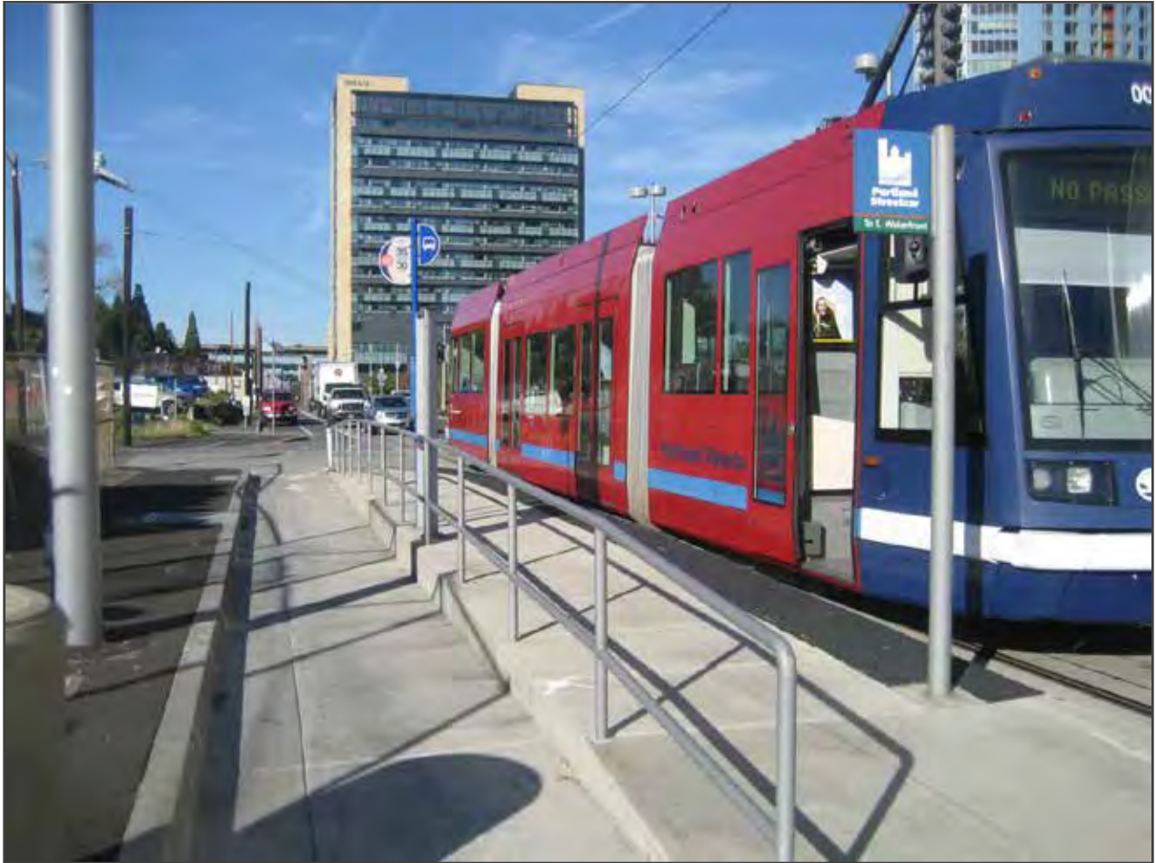
Figure 32: Example of a Bike Lane at a Stop Island in Portland
