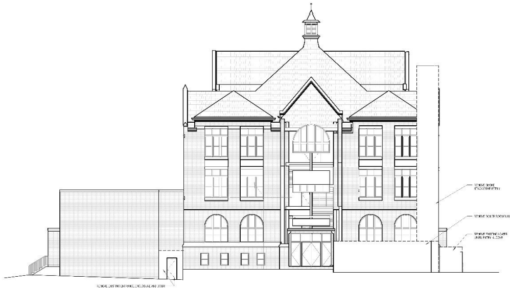
2 NORTH DEMOLITION ELEVATION SCALE: 1/8" = 1'-0"
