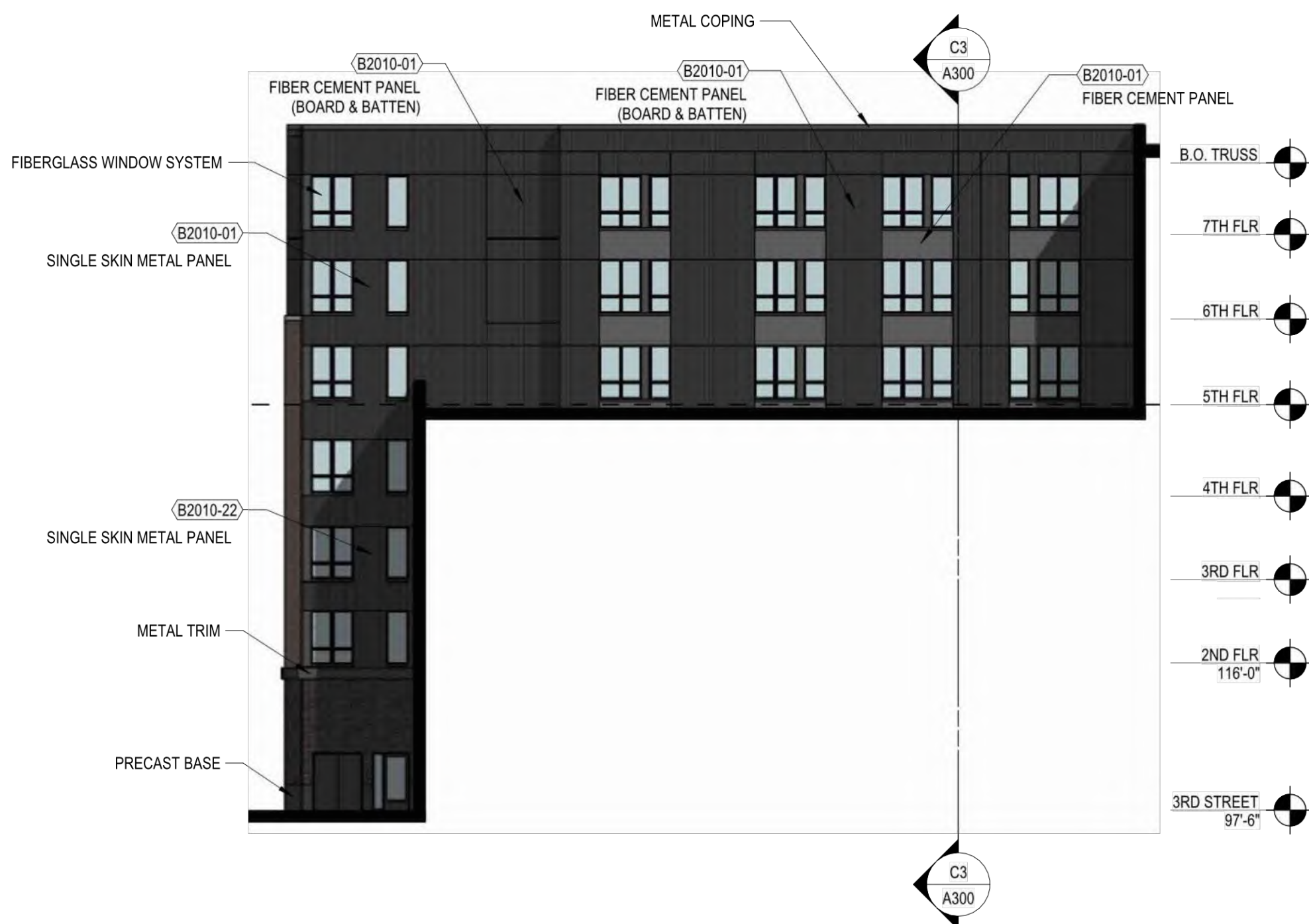
C4 WEST ELEVATION - COURTYARD 1/16" = 1'-0" | A202
