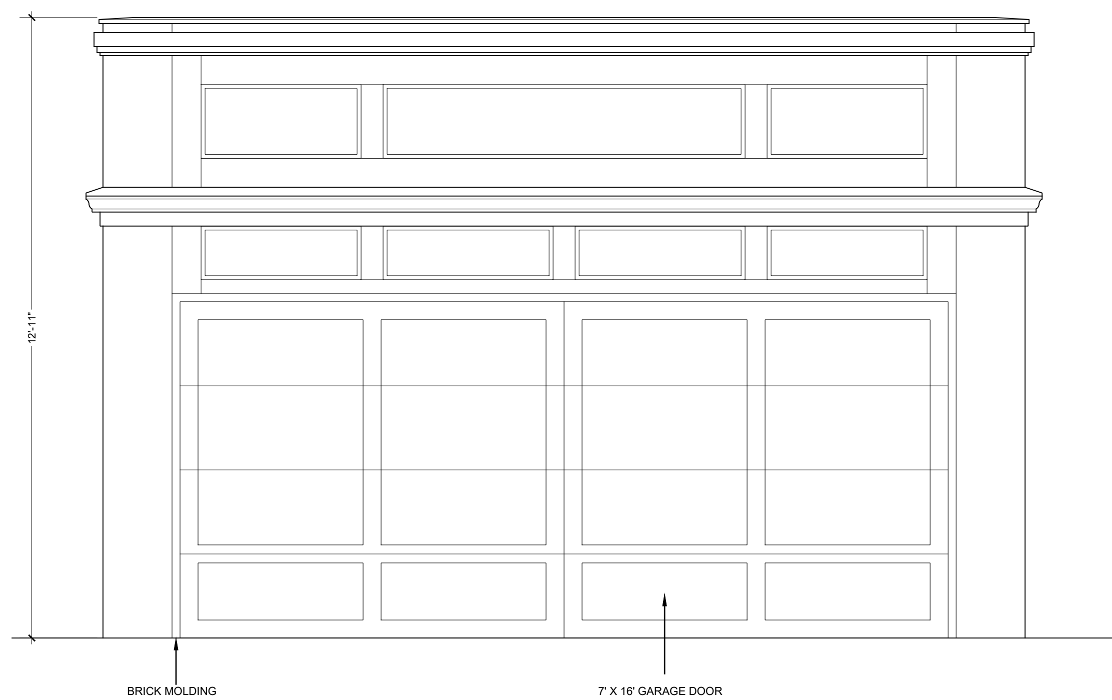
3 SOUTH ELEVATION (FRONT) 1/2" = 1'-0"
