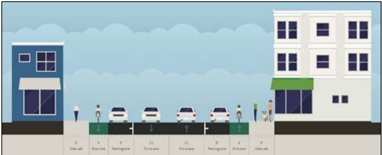
Image 1: Conceptual image of North 27th Street cross section with bike lanes buffered by the parking lane. Credit: Streetmix.com
