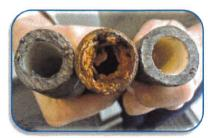
Left to right: A lead pipe, a corroded steel pipe, and a lead pipe with protective coating.
