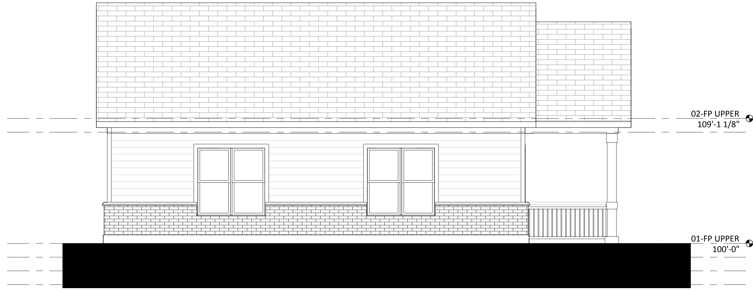
4 COMMUNITY BLDG NORTH ELEVATION SCALE: 1/4" = 1'-0"
