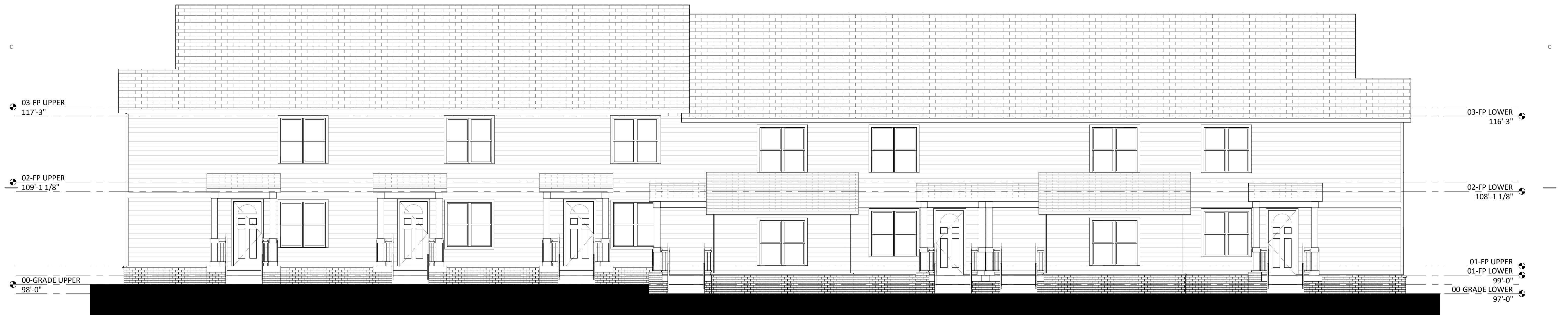
2 7 UNIT BLDG SOUTH ELEVATION SCALE: 3/16" = 1'-0"
