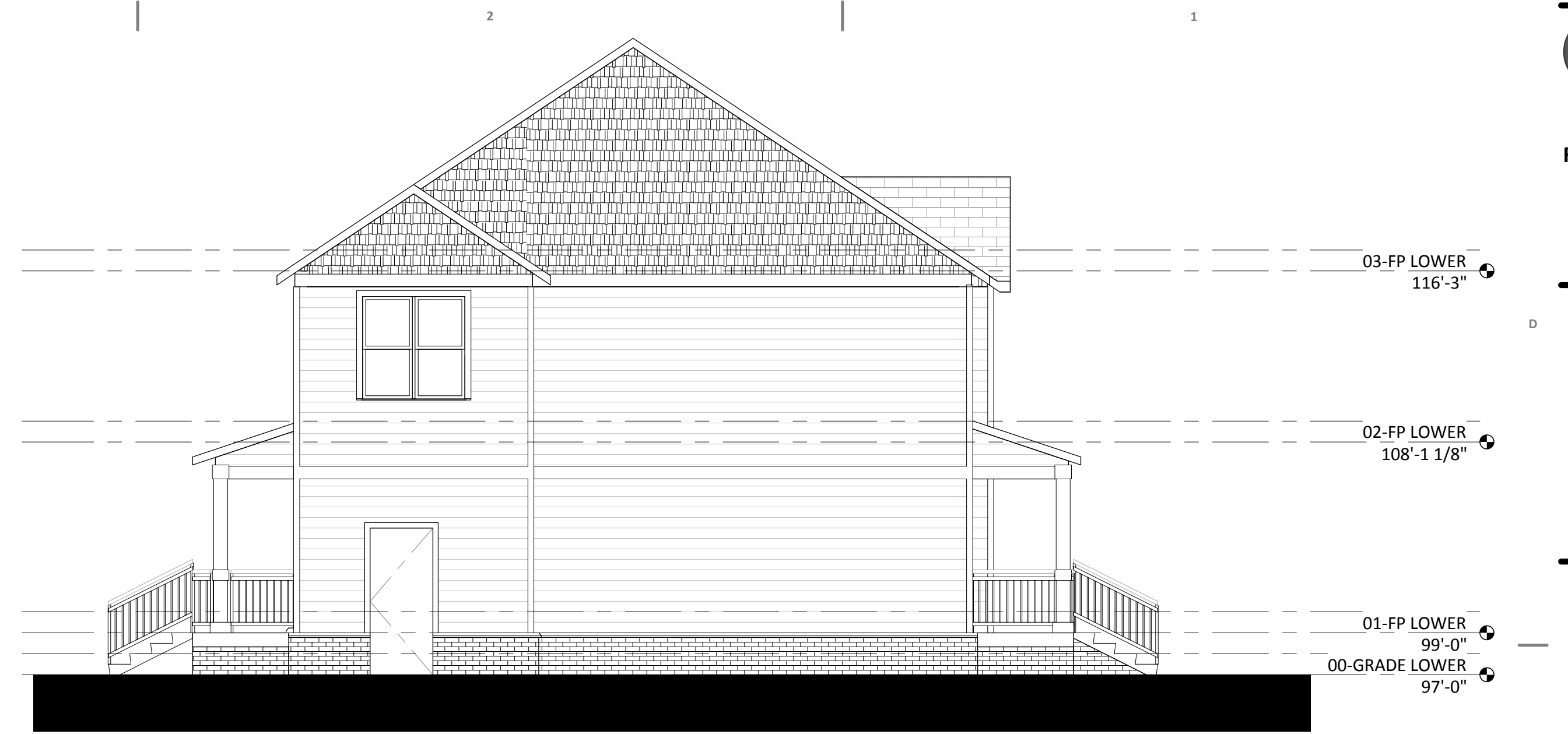
3 6 UNIT BLDG EAST ELEVATION SCALE: 3/16" = 1'-0"
