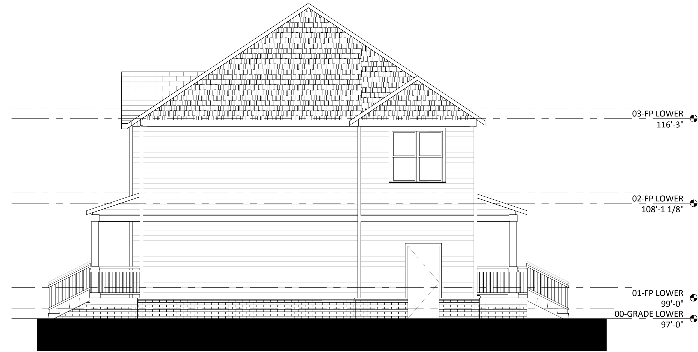
4 10 UNIT BLDG SOUTH ELEVATION SCALE: 3/16" = 1'-0"
