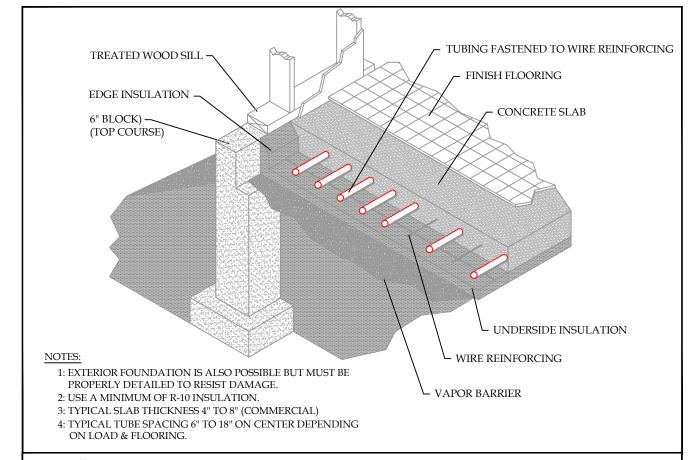
$\underline{\mathsf{IMC}\,\mathsf{1208.1}}\,\mathsf{-HYDRONIC\,PIPING\,SYSTEMS}, \mathsf{OTHER\,THEN\,GROUND\,SOURCE\,HEAT\,PUMP\,LOOP\,SYSTEMS},$ SHALL BE TESTED HYDRONICALLY AT 1-1/2 TIMES THE MAXIMUM SYSTEM DESIGN PRESSURE, BUT NOT LESS THAN 100 PSI. THE DURATION OF EACH TEST SHALL BE NOT LESS THAN 15 MINUTES. GROUND SOURCE HEAT PUMP LOOP SYSTEMS SHALL BE TESTED PER IMC 12081.1
