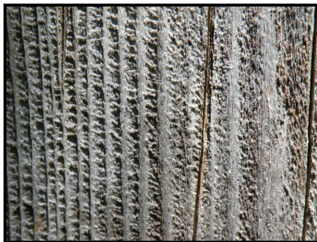
Figure 4.3. Detail of an uncoated wood substrate with erosion of the earlywood due to weathering.
