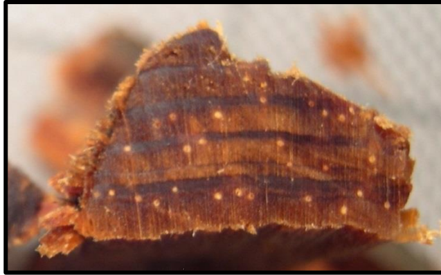
Figure 2.1. Cross section (end grain) of southern yellow pine, showing dark latewood bands.
