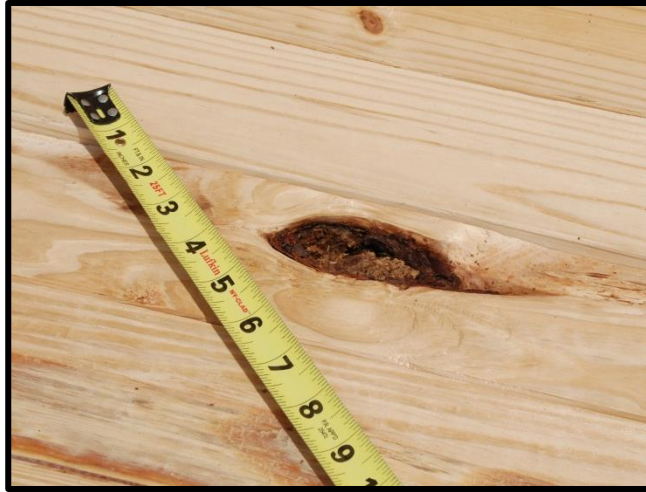
Figure 2.6. Bark Inclusions occur when a bark-covered branch or a separate stem becomes incorporated into the main trunk.
