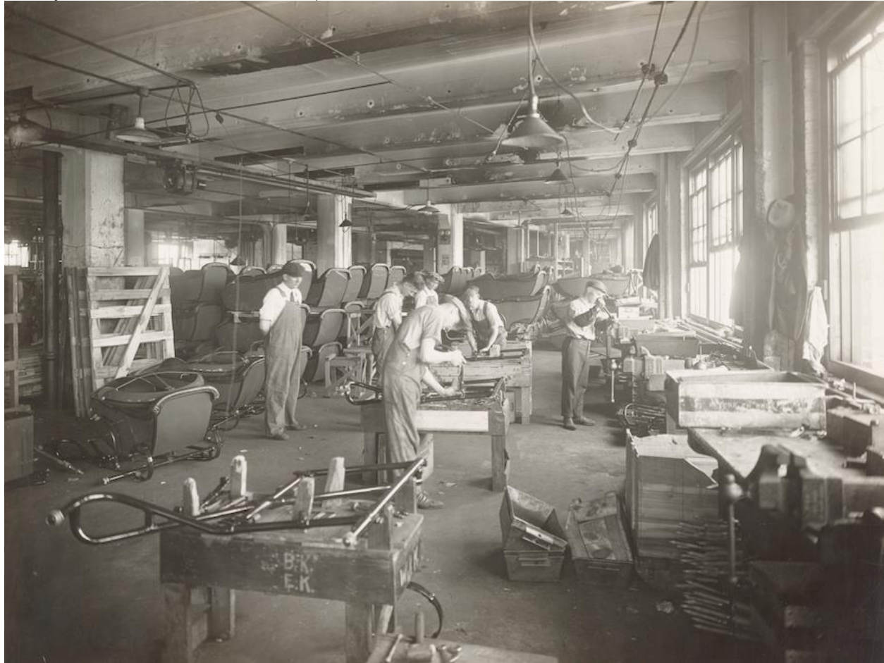
Figure 15. Interior photo of frame manufacturing within the 3700 Building c. 1912. (Courtesy Harley-Davidson Museum Archive)
