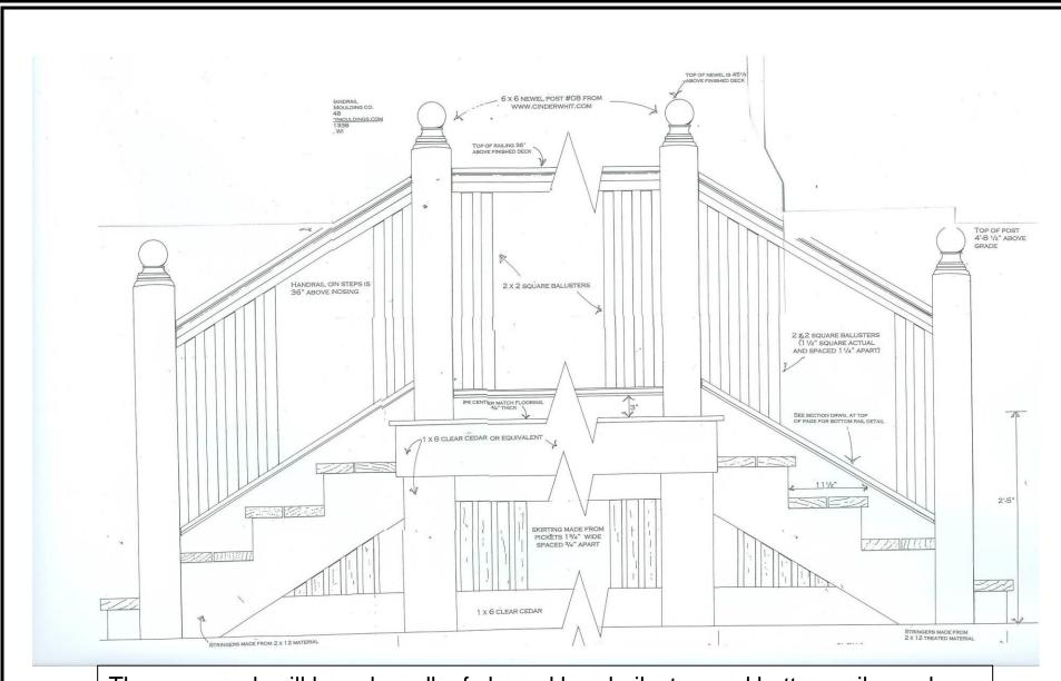
The new porch will have breadloaf shaped handrails, tapered bottom rails, and square picket balusters spaced 1½ inch apart. Porch steps will meet code and skirting will be simple boards as shown above.
