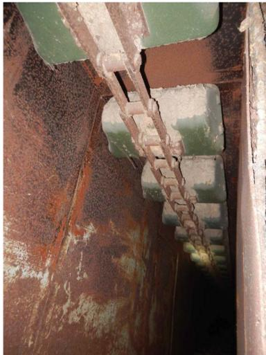
(K4) INTERIOR DETAIL OF THE GRAIN ELEVATOR SHOWING THE CONTAINERS AND CONVEYOR SYSTEM TO BE DISPLAYED THRU THE EXISTING HATCH DOORS.
