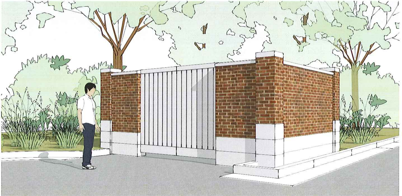
MASONRY SCREEN WALL TRASH ENCLOSURE
