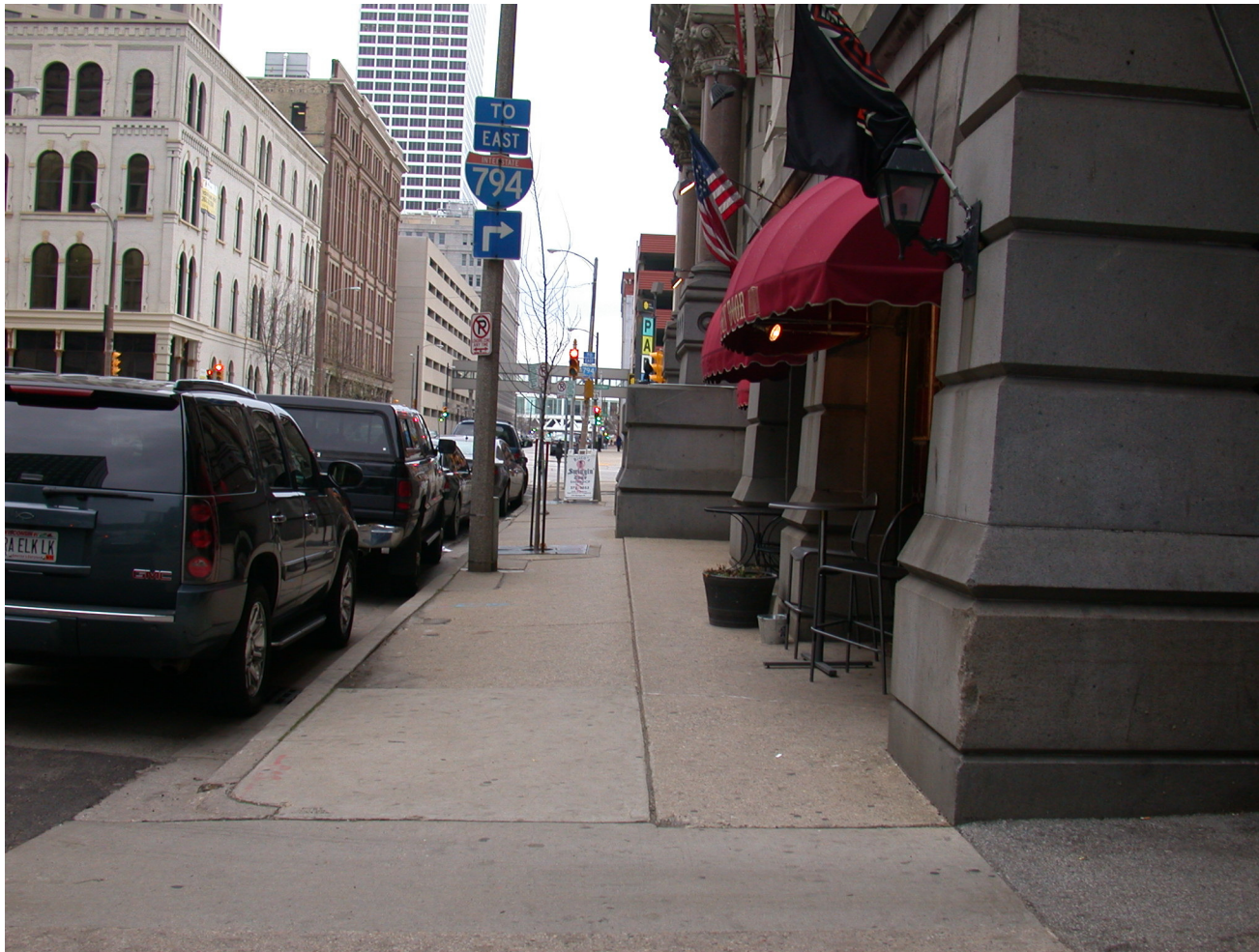
CCF 091220 225 East Michigan Street 11-29-2010 Looking east towards North Broadway at south sidewalk area of Michigan Street. Note: There is a 5-foot clear path for pedestrians around the encroachments.
