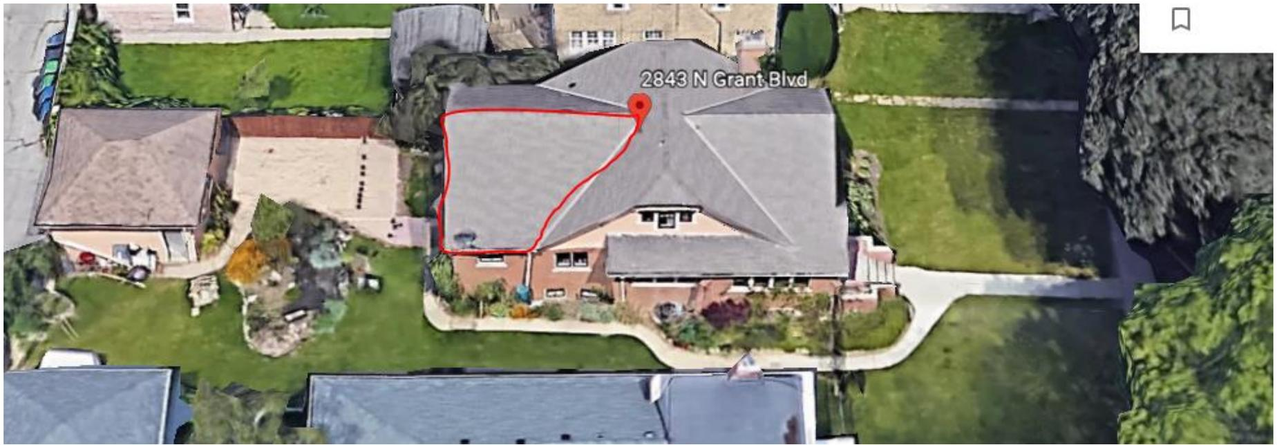
Solar panels are approved for installation only on the roof slope outlined in red. Required electrical equipment shall be installed on the rear (west) wall or the building interior.
