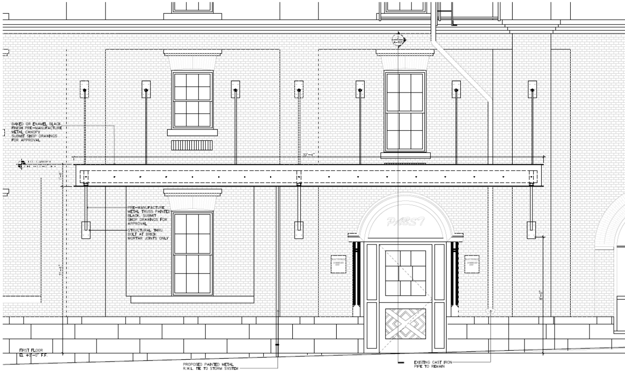
1 PARTIAL BUILDING ELEVATION PROPOSED ENTRANCE CANOPY SCALE: 1/2" = 1'-0"
