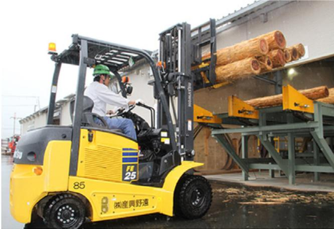
*FE25 Electric Forklift: FE-Series electric forklift trucks not only adopt easy-maintenance batteries and Komatsu-original rapid charging system, but also feature excellent water and dust-proof designs. As a result, FE-Series models can be used for handling heavy objects in demanding outdoor and dusty environments, where internal combustion models have conventional advantages over electric counterparts.*
