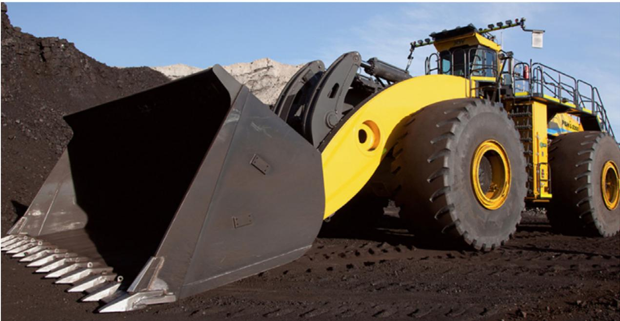
*P&H-brand L-2350 wheel loader features the standard bucket capacity of 40.52m<sup>3</sup>, about doubling that of KOMATSU-brand WA1200 wheel loader, the largest model conventionally offered by Komatsu.*
