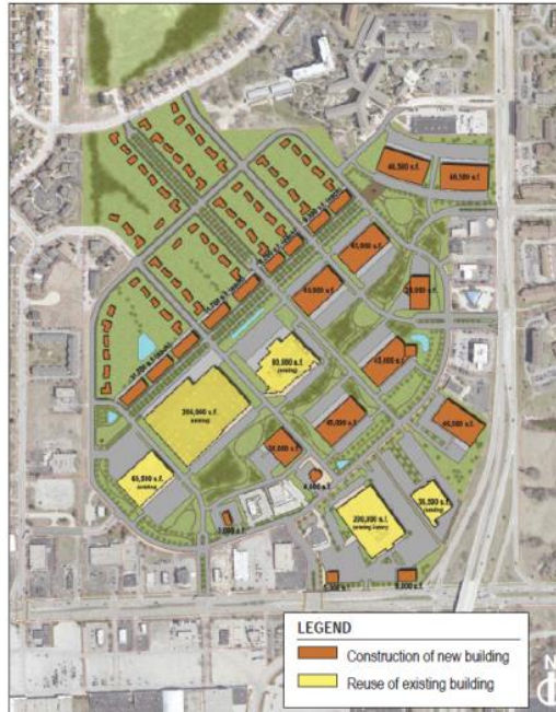
Figure 6. Conceptual site plan for the former Northridge Shopping Center (Option C).
