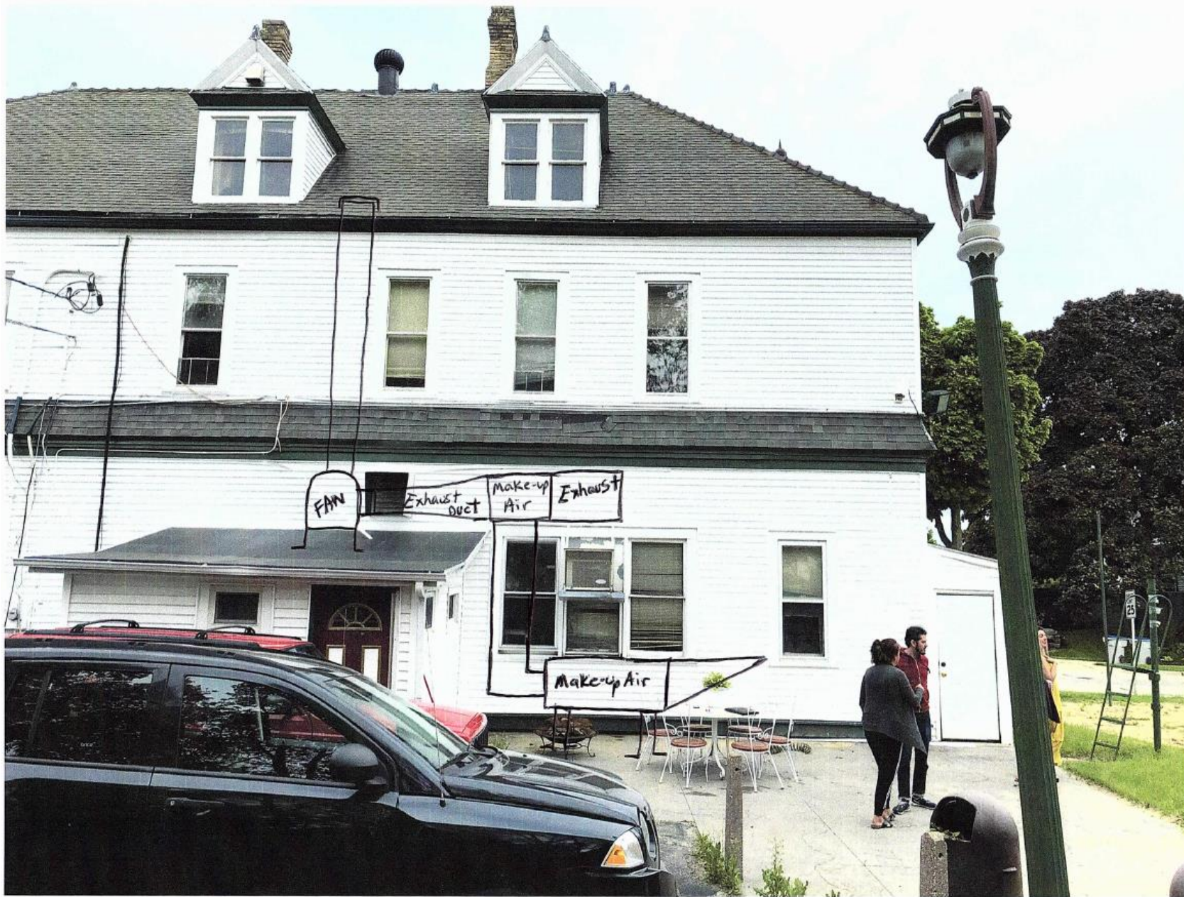
Elevation sketch of the exhaust and make-up air duct work to be completed
