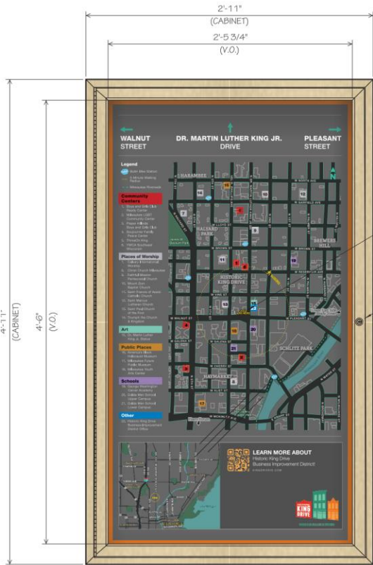
1 DISPLAY CABINET DETAIL - PS-1 1-1/2" = 1'-0" SCALE
