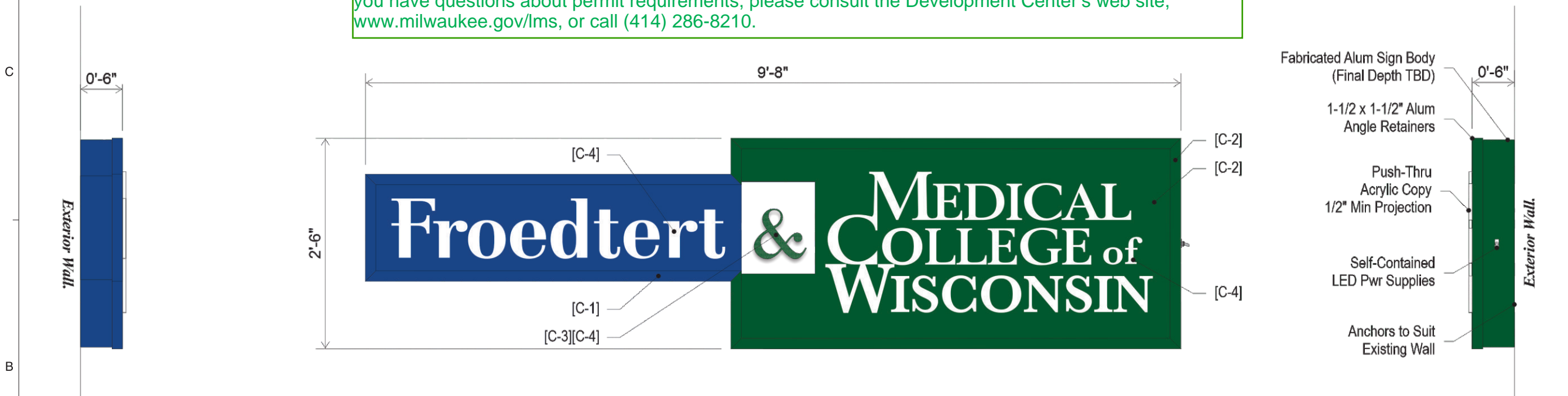
1 S/F Face-Lit, Push-Thru Acrylic ID Sign - 24SF P_01 (x3) Req'd 3/4" = 1' - 0" Scale
