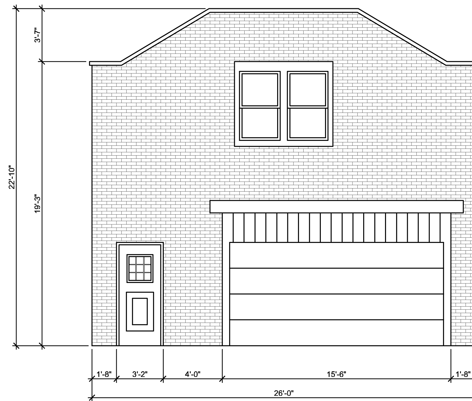
COACH HOUSE EXISTING NORTH ELEVATION 1/4" = 1'-0"
