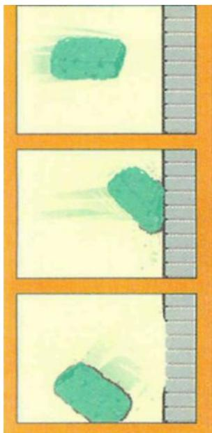
In sponge blasting, stone ornaments, statues, balustrades, columns, walls, stair treads and the dome were bombarded with tiny sponges shot pneumatically. They flatten on impact and grab the dirt before falling. Source: Sponge-Jet INC
