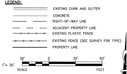
**NOTE:** EXISTING UTILITIES SHOWN ARE INDICATED IN ACCORDANCE WITH AVAILABLE RECORDS AND FIELD MEASUREMENTS. THE CONTRACTOR SHALL BE RESPONSIBLE FOR OBTAINING EXACT LOCATIONS AND ELEVATIONS OF ALL UTILITIES, INCLUDING SEWER AND WATER FROM THE OWNERS OF THE RESPECTIVE UTILITIES. ALL UTILITY OWNERS SHALL BE NOTIFIED BY THE CONTRACTOR 72 HOURS PRIOR TO EXCAVATION.
