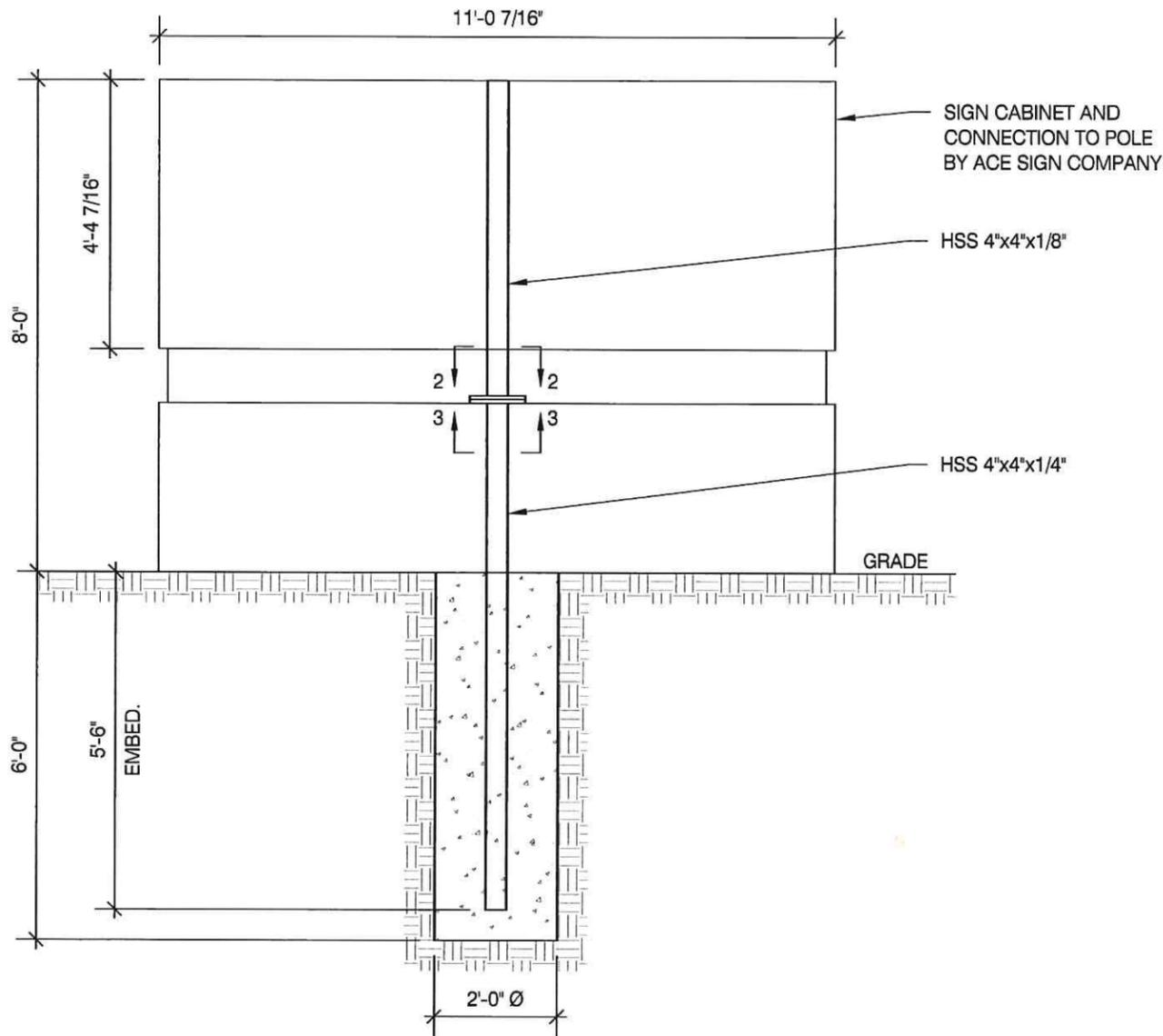
FRONT ELEVATION W/ CAISSON FOUNDATION
