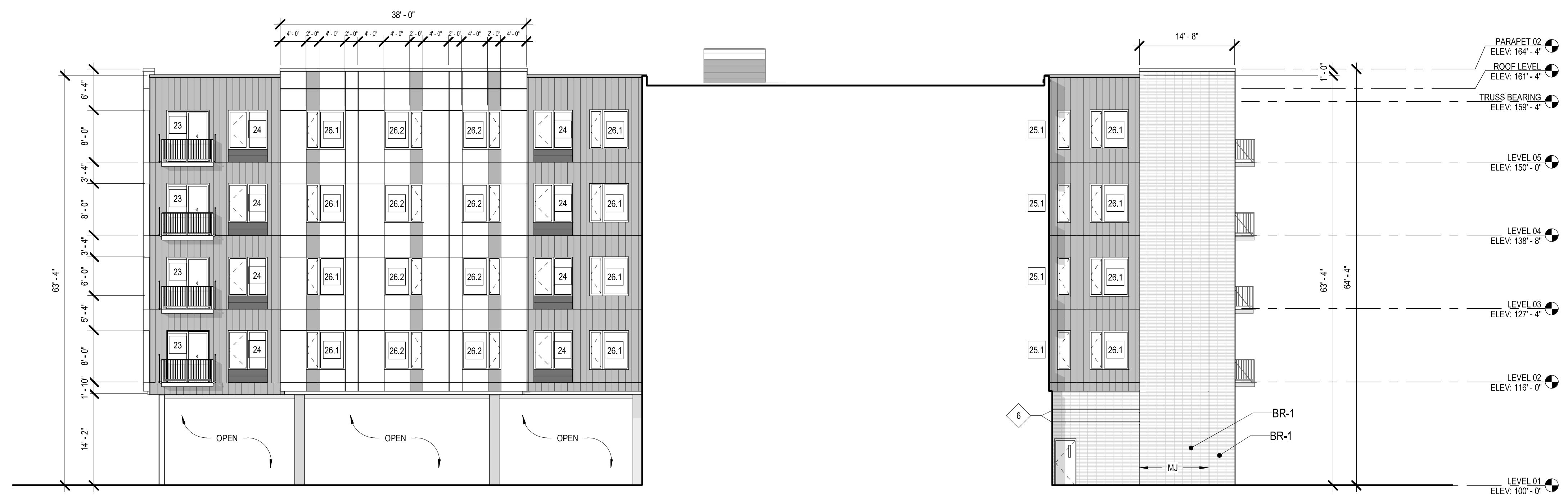
2 NORTH SECTION-ELEVATION THROUGH CENTRAL SPINE F11 - F3 Scale: 3/32" = 1'-0" 0' 1" 2" 4" 6"
