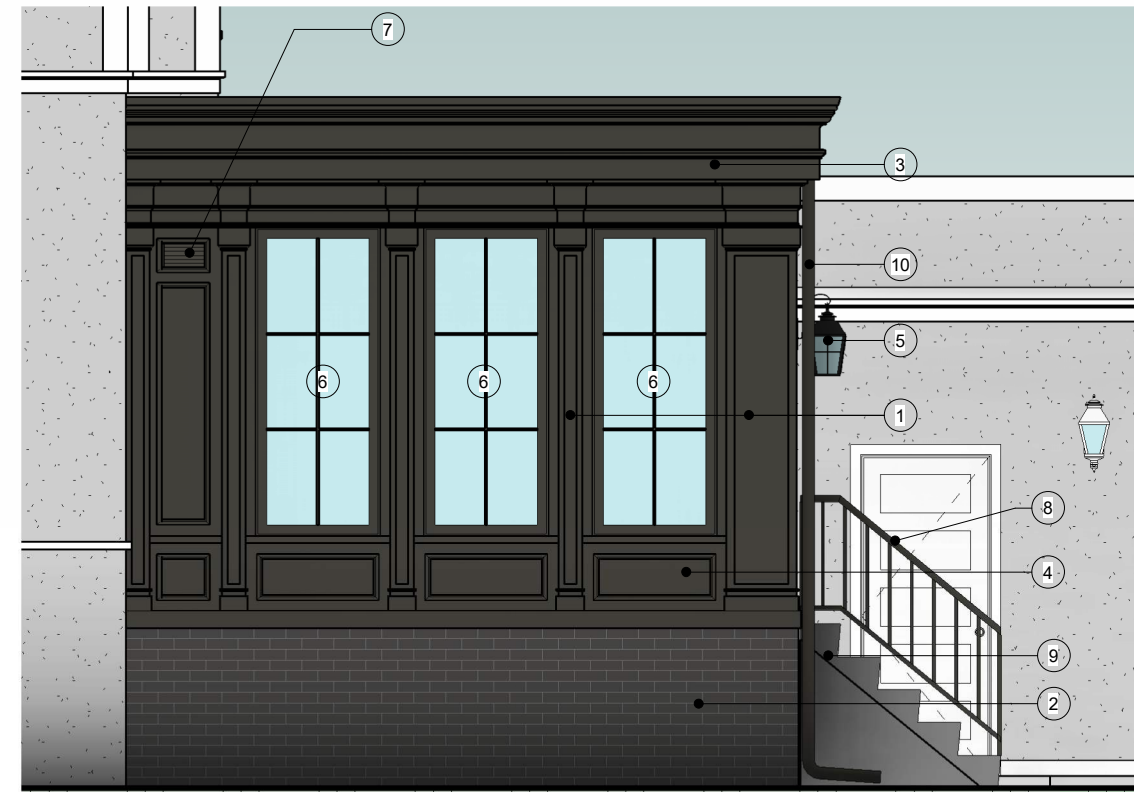
3 West Elevation - Addition 1/4" = 1'-0"
