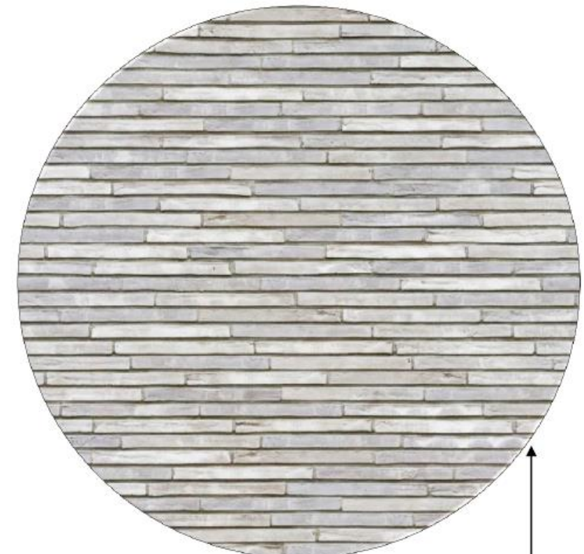
MASONRY VENEER 1 SIZE 2 1/4" x 16"
