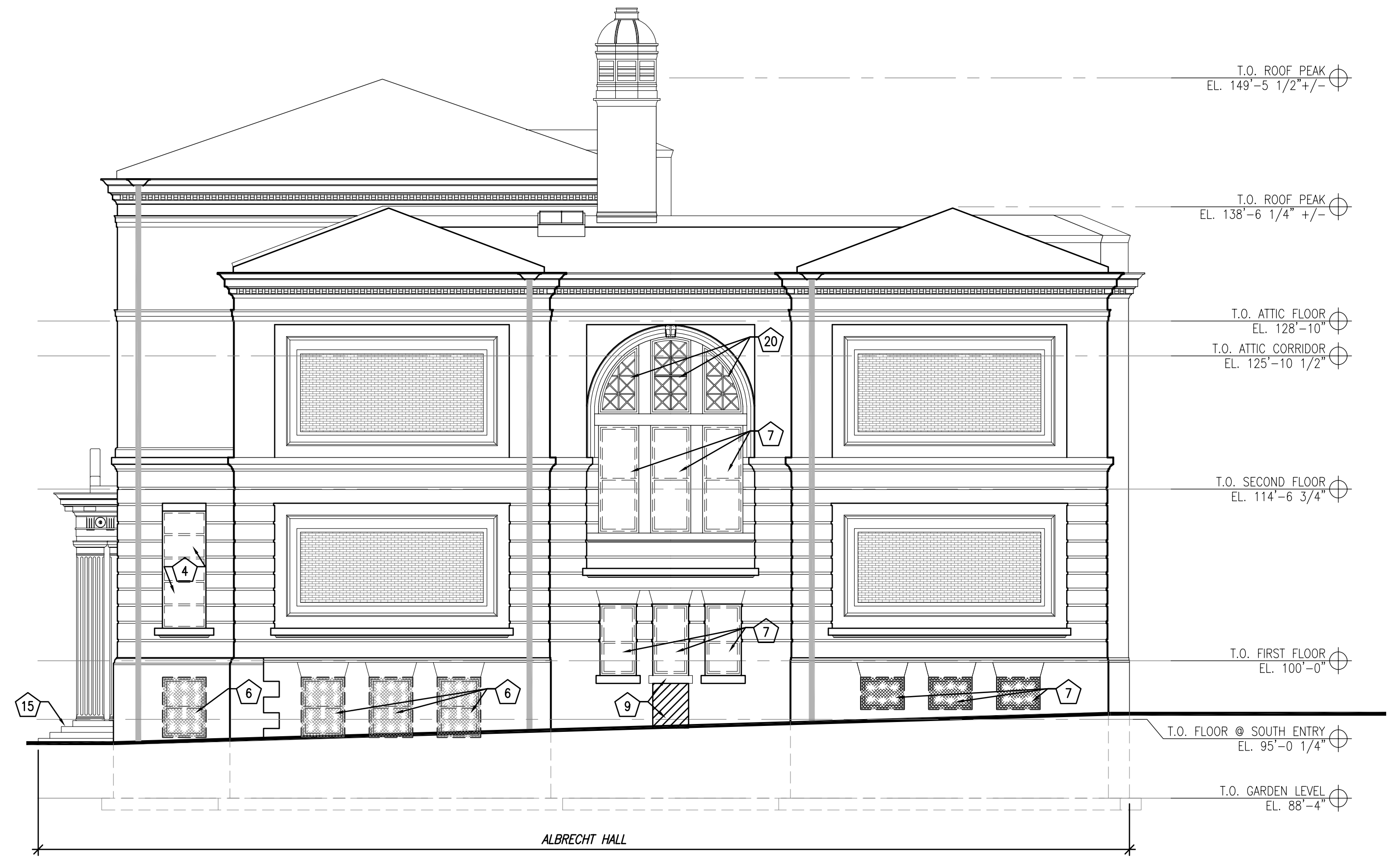
2 EAST BUILDING ELEVATION (DEMOLITION) SCALE: 1/8" = 1'-0"
