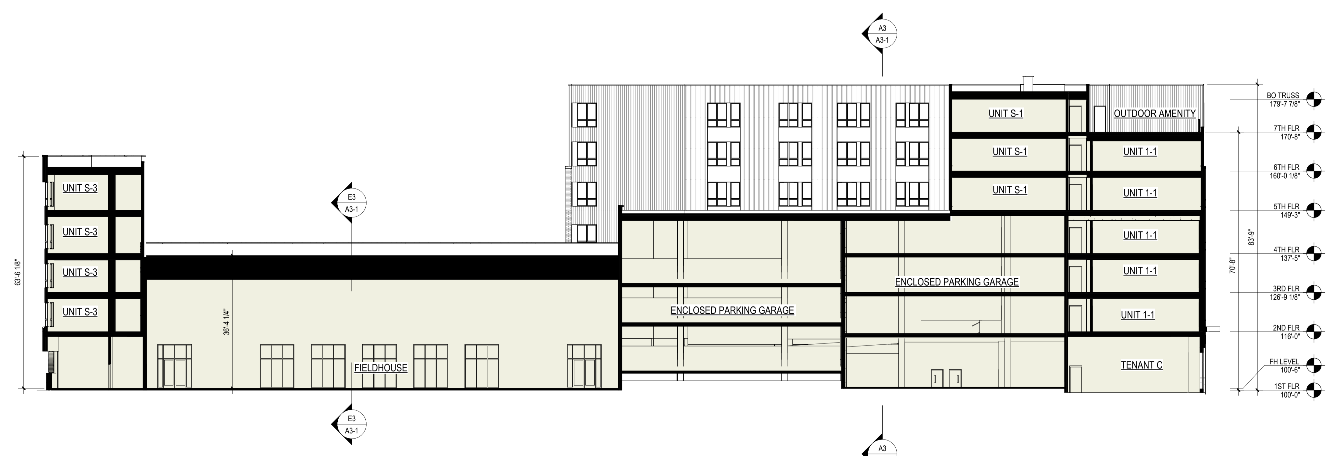
C3 BUILDING SECTION - N/S 1/16" = 1'-0" | A3-1
