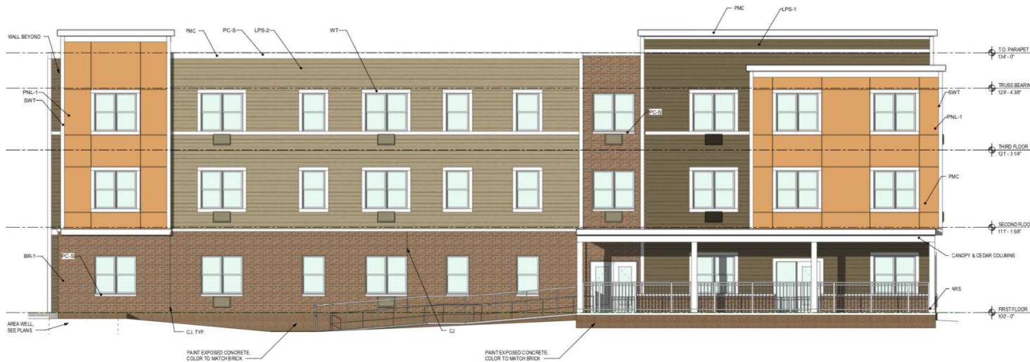
1 EXTERIOR ELEVATION - NORTH 3/16" = 1'-0"
