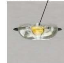
Micro-reflector behind LED enhances forward throw and reduces backlight
