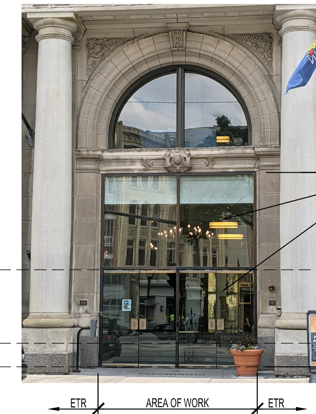
4 PARTIAL NORTH ELEVATION - DEMOLITION 1/8" = 1'-0"
