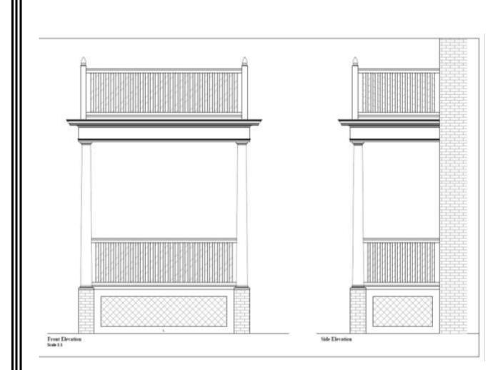
Rebuild to drawings with red cedar finish wood over PT-structure. Will use same railing design for front balcony
