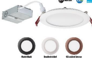
WF6 LED 40K, 4000 K LEDs, Input watts: 13.6, delivered lumens: 1200, LM/W=88.2, test no. ISF 30295
