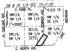
All bearings are referenced to the Wisconsin State Plane Coordinate System (South zone) dated Dec., 2012 in which the South line of the SW 1/4, Sec. 15 bears N88°51'30"E. Tax Key: 3180081110 & 3180081120 -See Sheet 2 for Lot 1 details
