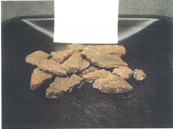
USHG 12-006A Exterior Iron Spot Face Brick mortar, Butterjoint
