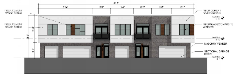
2 BUILDING B - WEST ELEVATION
