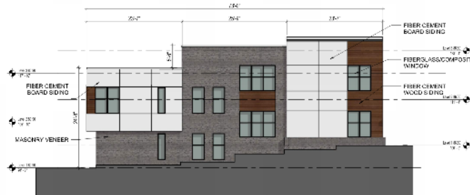
3 BUILDING B - NORTH ELEVATION
