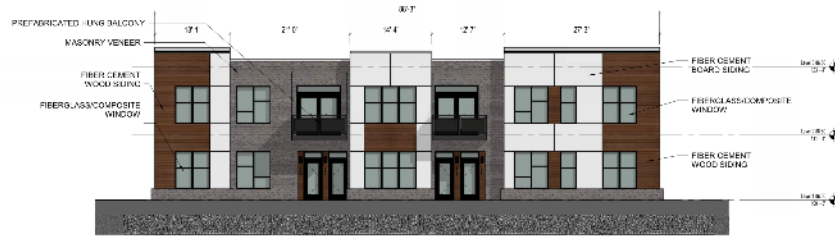
1 N. PALMER ST. ELEVATION - BUILDING B
