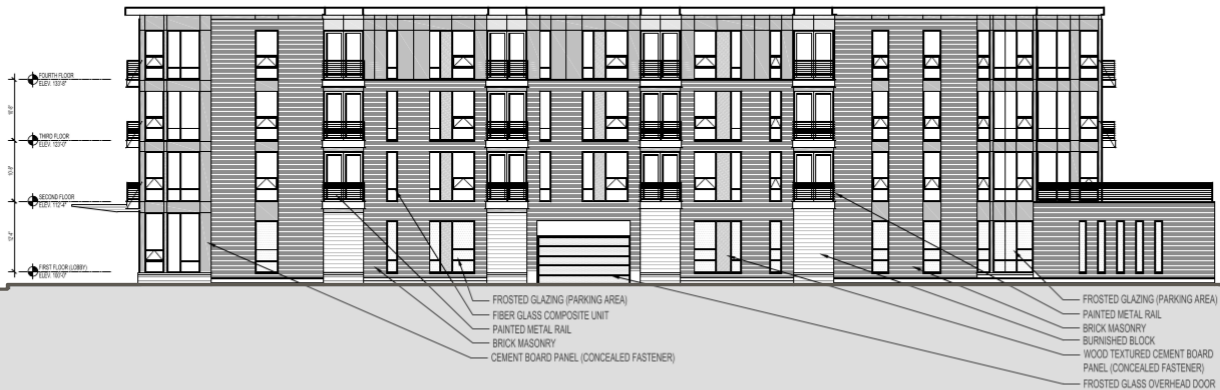
BUILDING 1 WEST ELEVATION SCALE: 1/8"=1'-0"
