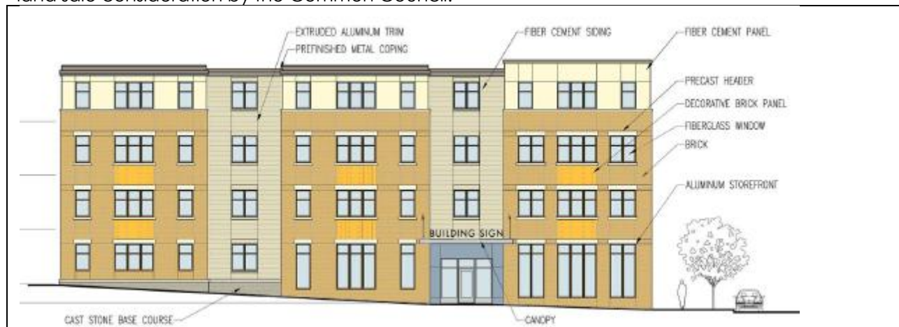
Center Street Elevation
